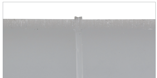
Lateral cut of IR (infrared) welding
