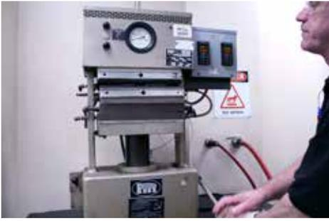
3 Next, the resin is heated and pressed to flatten the material to under 1/10 of an inch with several tons of pressure. This is used to check for correct color using a color platen.
