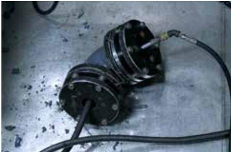
9 Fittings are routinely pressure-tested to failure. This process helps us understand safety factors and ensures the fitting meets or exceeds ASTM standards.
