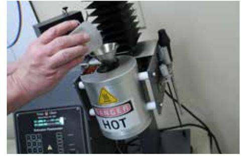
5 After color check, the melt flow indexer is used to measure the viscosity of the material and how it will behave in the molding and extrusion processes. If the material passes this final step, it can then be released to production.
