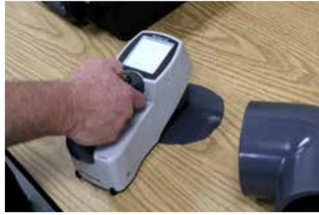
4 It is then analyzed using the color spectrometer. If the material's color is out of tolerance and does not meet specification, the material is rejected.
