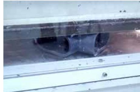
10 In addition to pressure tests, fittings are also crushed under extreme pressures. ASTM requires a 25% compression in order to pass. A GF fitting will usually meet a 75% or better compression without fracture. Fittings that pass this test are considered ductile and will not fail catastrophically.
