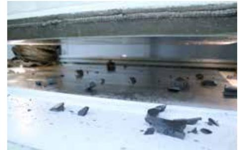
11 Although some fittings may look similar, they don't all behave the same. At GF, we often analyze and compare competitors' fittings to ours. Here is an example of a competitor's fitting during the crush test resulting in a catastrophic failure.
