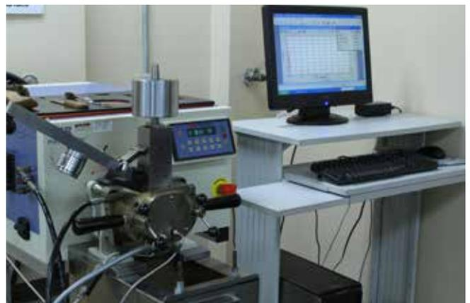
2 Once preliminary checks are complete, the resin is checked with a Brabender or torque rheometer that simulates the way the material will behave when processed through molding machines and extruders. If raw material is out of specification, it will be rejected at this time.
