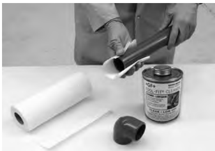
Cleaning the pipe and socket
