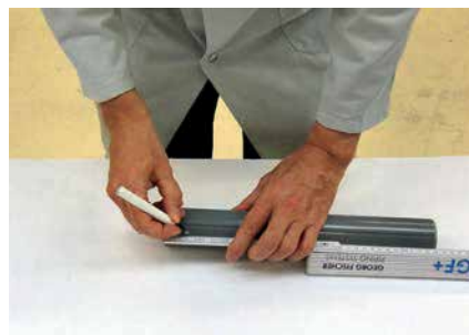
Marking the joining length
