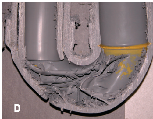
14 days: failed pressure check, no liquid left
